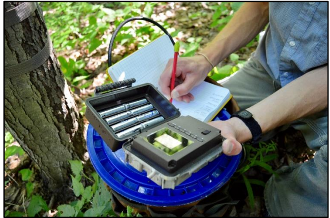
Figure 70. Retrieving SD cards from the field and capturing metadata.
